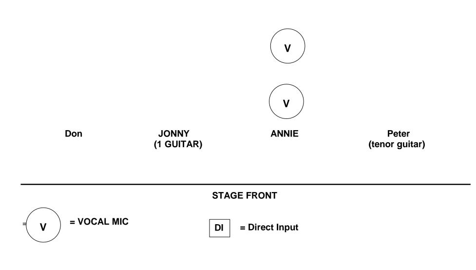
For a small room we definitely prefer using two omni directional mikes for all sound reinforcement. Both mikes are placed centrally in front of Annie. One is mainly for vocals and the 2<sup>nd</sup> one is lower to pick up the instruments.
